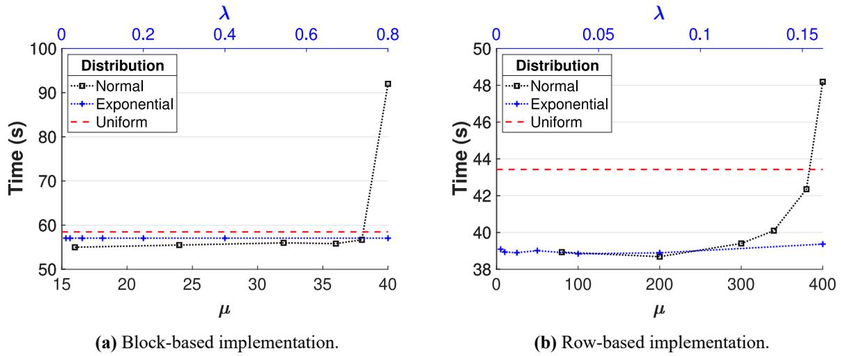
**Figure 18.** Wahab calculation times for each implementation and all three distributions. Note the  $\lambda$ -labeled axis pertains to the exponential distribution trajectory while the  $\mu$ -labeled axis refers to the normal distribution trajectory.
